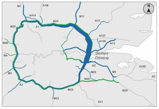
Blue shows a reduction in flow and green shows an increase in flow compared to the normal operation FIGURE 4.15 - FLOW REDUCTION AS A RESULT OF CLOSING A TUNNEL AT DARTFORD IN 2025 (WITHOUT SCHEME)
