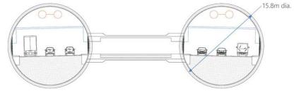
FIGURE 8.3 - INDICATIVE DUAL 3 LANE BORED TUNNEL CROSS SECTION
