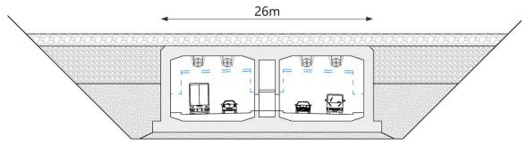
FIGURE 5.13 - IMMERSED TUNNEL CROSS SECTION AT LOCATION C
