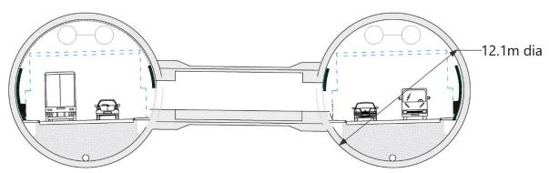
FIGURE 5.12 - BORED TUNNEL CROSS SECTION AT LOCATION C
