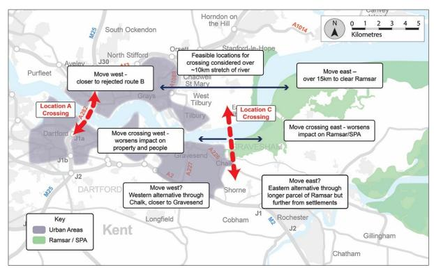
FIGURE 5.8 - DETERMINATION OF CROSSING POSITION AT LOCATION C
