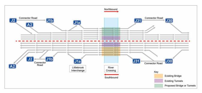
FIGURE 5.2 - ROUTE 1 SCHEMATIC LANE LAYOUT
