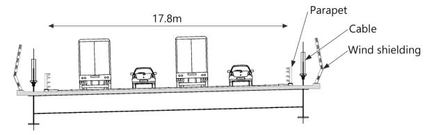
FIGURE 5.4 - BRIDGE CROSS SECTION AT LOCATION A
