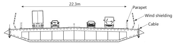
FIGURE 5.10 - BRIDGE CROSS SECTION AT LOCATION C
