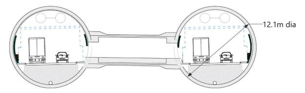
FIGURE 5.6 - BORED TUNNEL CROSS SECTION AT LOCATION A
