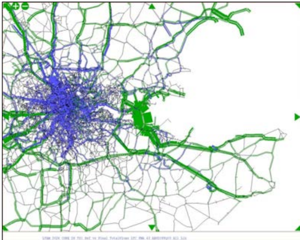
Figure 6.7 – Assigned Flow Differences – Reference Matrix Vs VDM Output Matrix (Core 2026 Reference Vs 2026 DS AM Peak)
