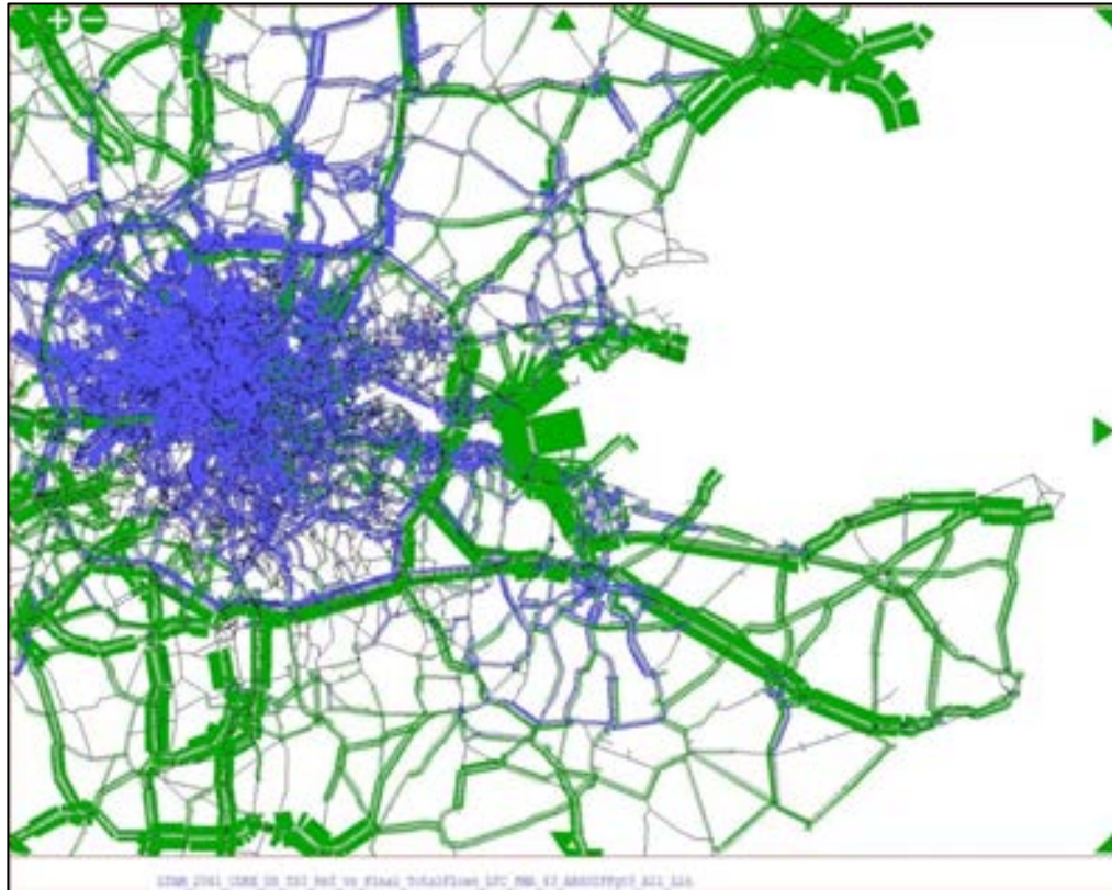
Figure 6.21 – Assigned Flow Differences – Reference Matrix Vs VDM Output Matrix (Core 2041 Reference Vs 2041 DS PM Peak)
