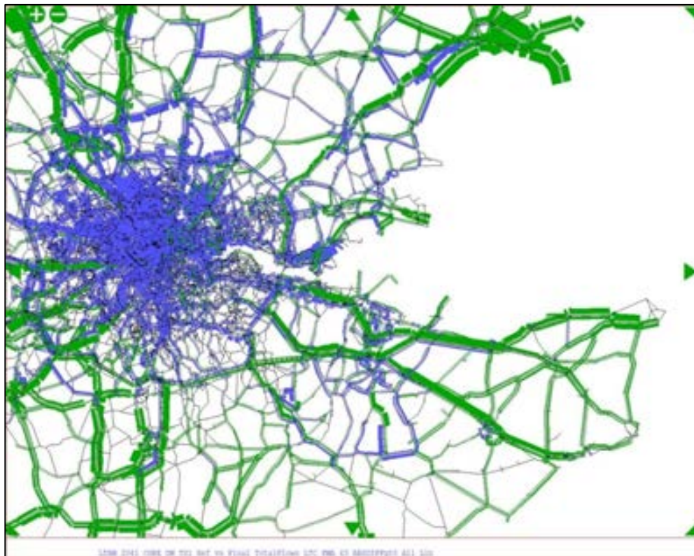
Figure 6.16 – Assigned Flow Differences – Reference Matrix Vs VDM Output Matrix (Core 2041 Reference Vs 2041 DM AM Peak)
