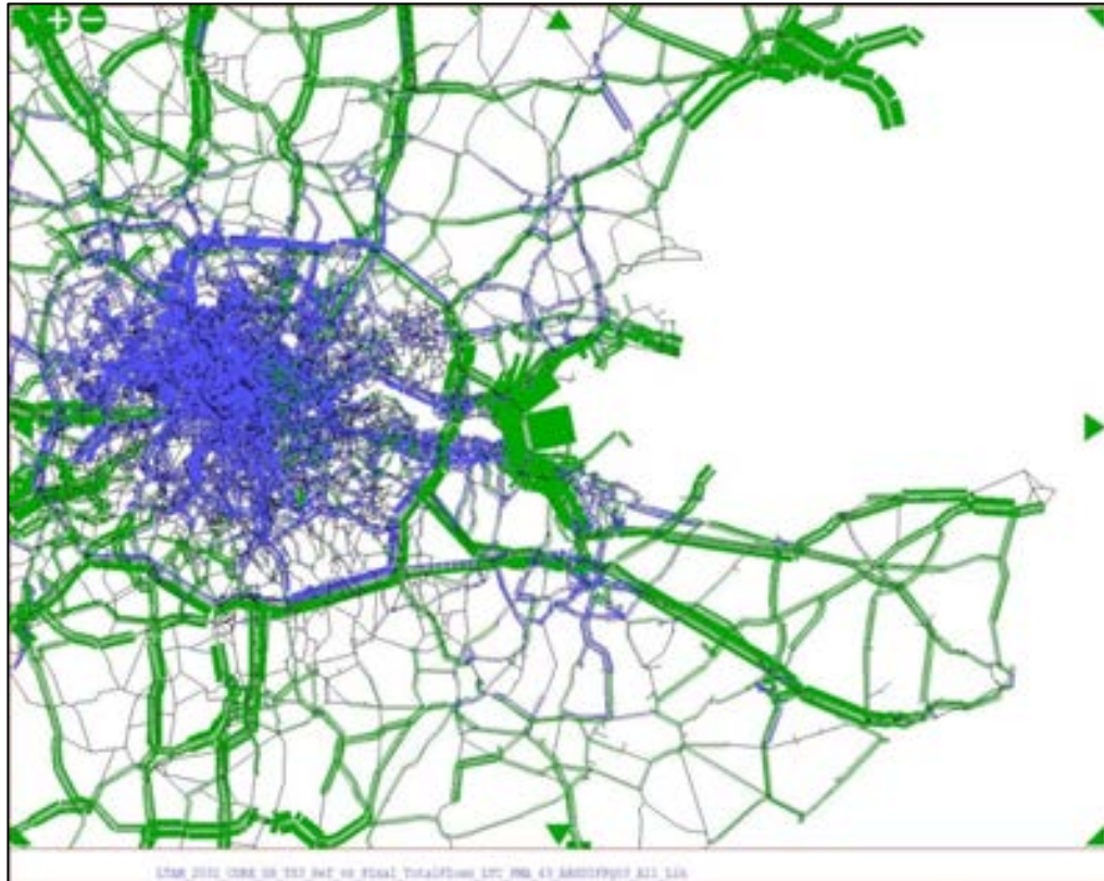
Figure 6.15 – Assigned Flow Differences – Reference Matrix Vs VDM Output Matrix (Core 2031 Reference Vs 2031 DS PM Peak)
