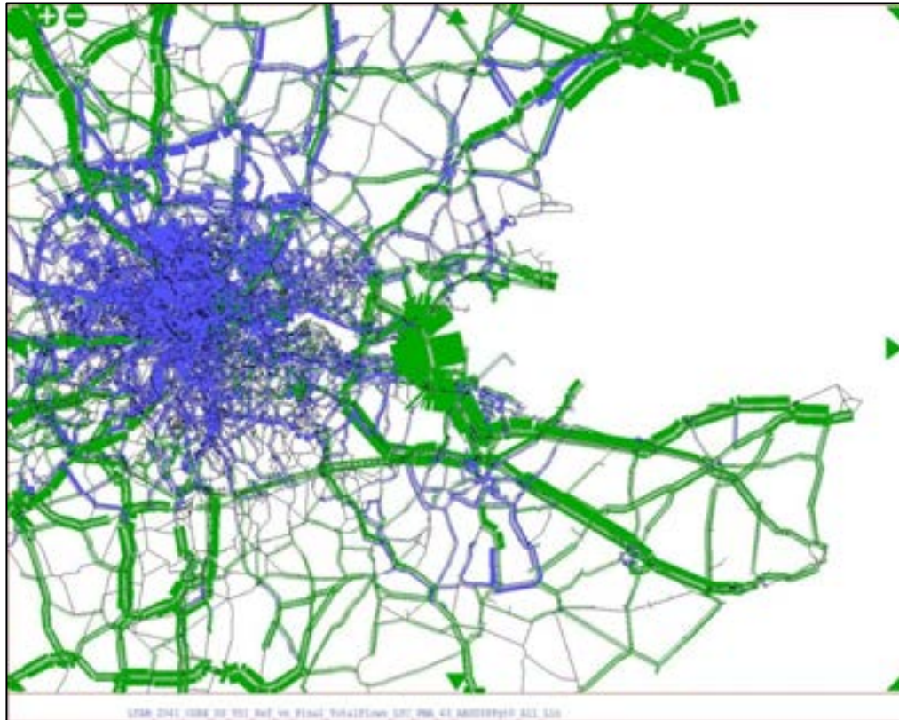
Figure 6.19 – Assigned Flow Differences – Reference Matrix Vs VDM Output Matrix (Core 2041 Reference Vs 2041 DS AM Peak)
