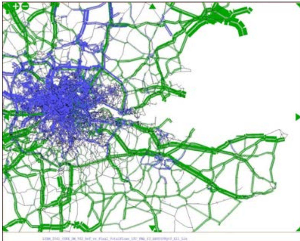
Figure 6.17 – Assigned Flow Differences – Reference Matrix Vs VDM Output Matrix (Core 2041 Reference Vs 2041 DM Inter Peak)
