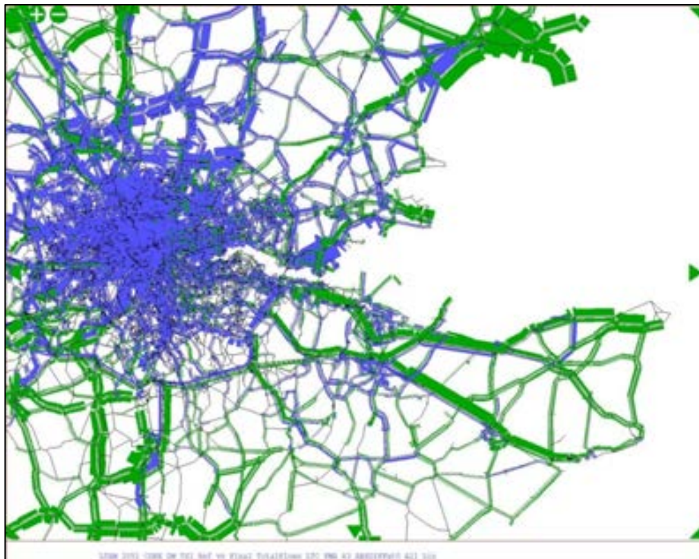
Figure 6.22 – Assigned Flow Differences – Reference Matrix Vs VDM Output Matrix (Core 2051 Reference Vs 2051 DM AM Peak)
