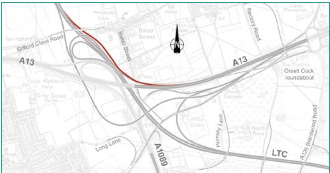
Figure 5-26. **LTC southbound to join the A13 eastbound, joins with the connection from LTC northbound (figure 5-25).** This connection will start in a cutting to pass under Stifford Clays Road before merging with the connection from the LTC northbound, passing over Baker Street and joining the A13
