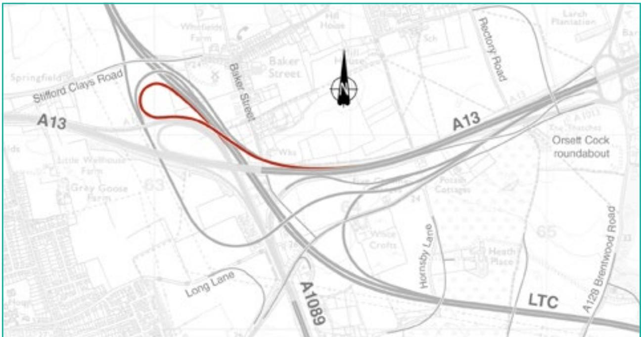
Figure 5-25. **LTC northbound to join the A13 eastbound.** This connection will start in a cutting before rising to cross the LTC and merge with the connection from the LTC southbound on an embankment, passing over Baker Street and joining the A13
