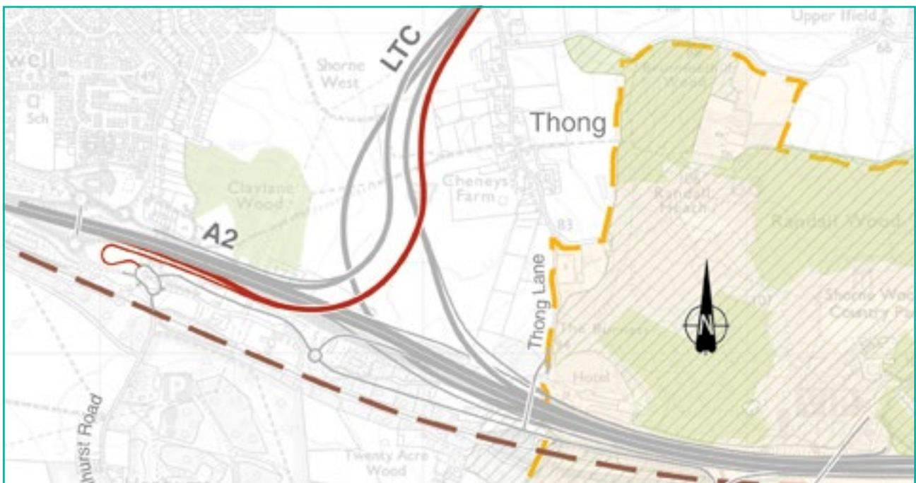
Figure 5-2. **Leaving the LTC to join the A2 westbound.** Also connects to the Gravesend east junction, where the existing slip road will no longer connect to the A2. The road will pass over the LTC, the M2/A2 westbound to the LTC northbound and the A2 main road
