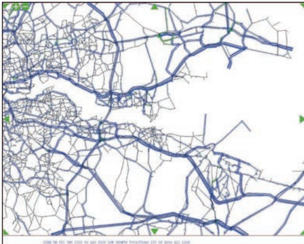
Figure E1 – Flow Difference Plot – Low Growth Scenario Minus Core Scenario 2026 DM AM Peak
