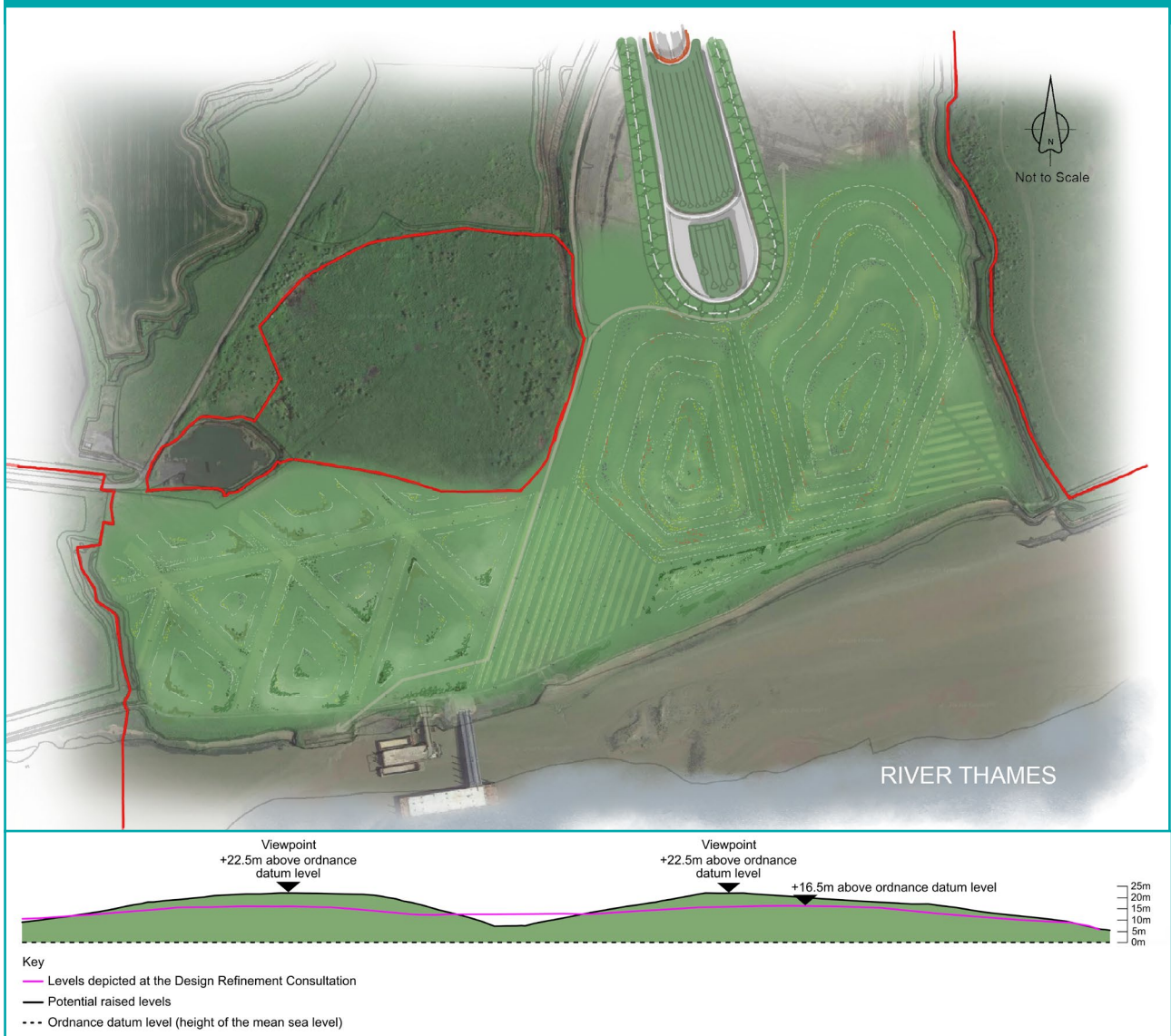
Figure 3-27 Proposed changes in the form and height of the earthworks at Tilbury Fields
