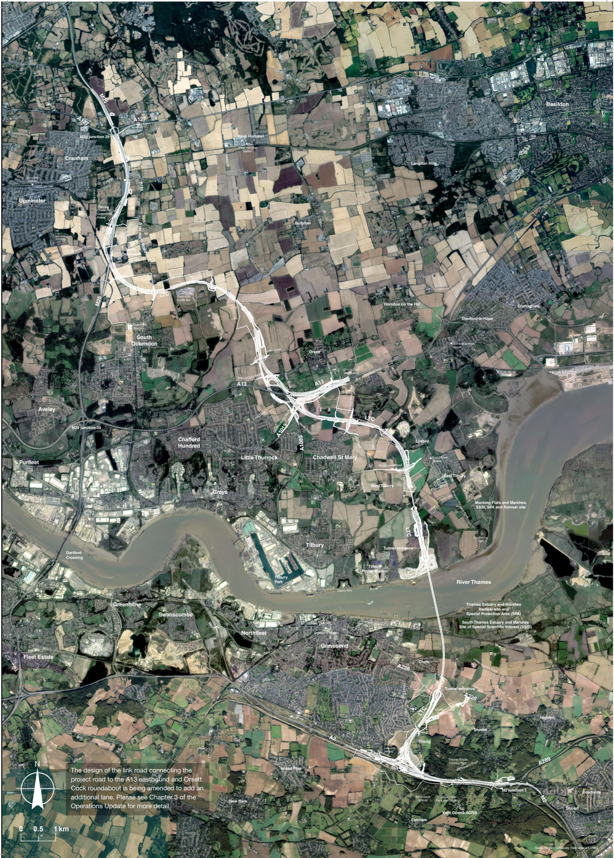
The design of the link road connecting the project road to the A13 eastbound and Orsett Cock roundabout is being amended to add an additional lane. Please see Chapter 3 of the Operations Update for more detail.
