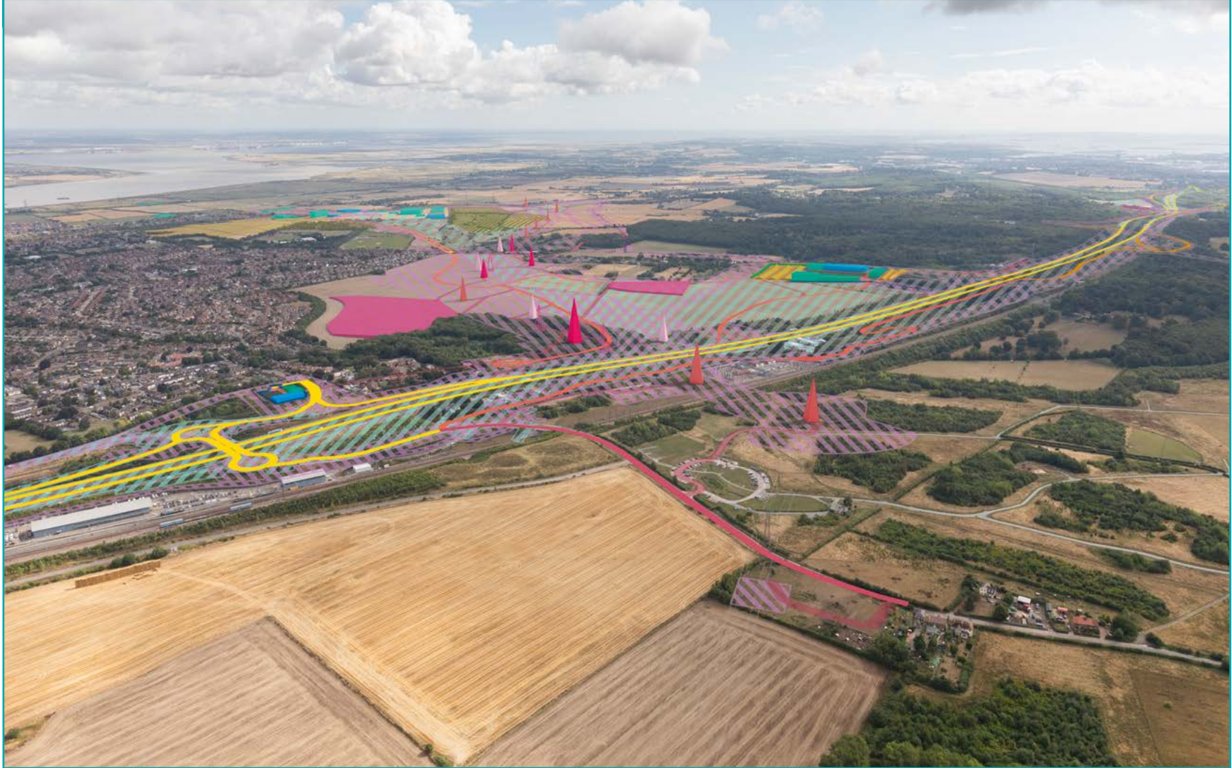
Figure 8-4 Indicative view during construction of the A2 corridor from west of Claylane Woods, looking north-east, showing the Marling Cross Compound, A2 West Utility Logistics Hub and combined utilities and highway construction areas
