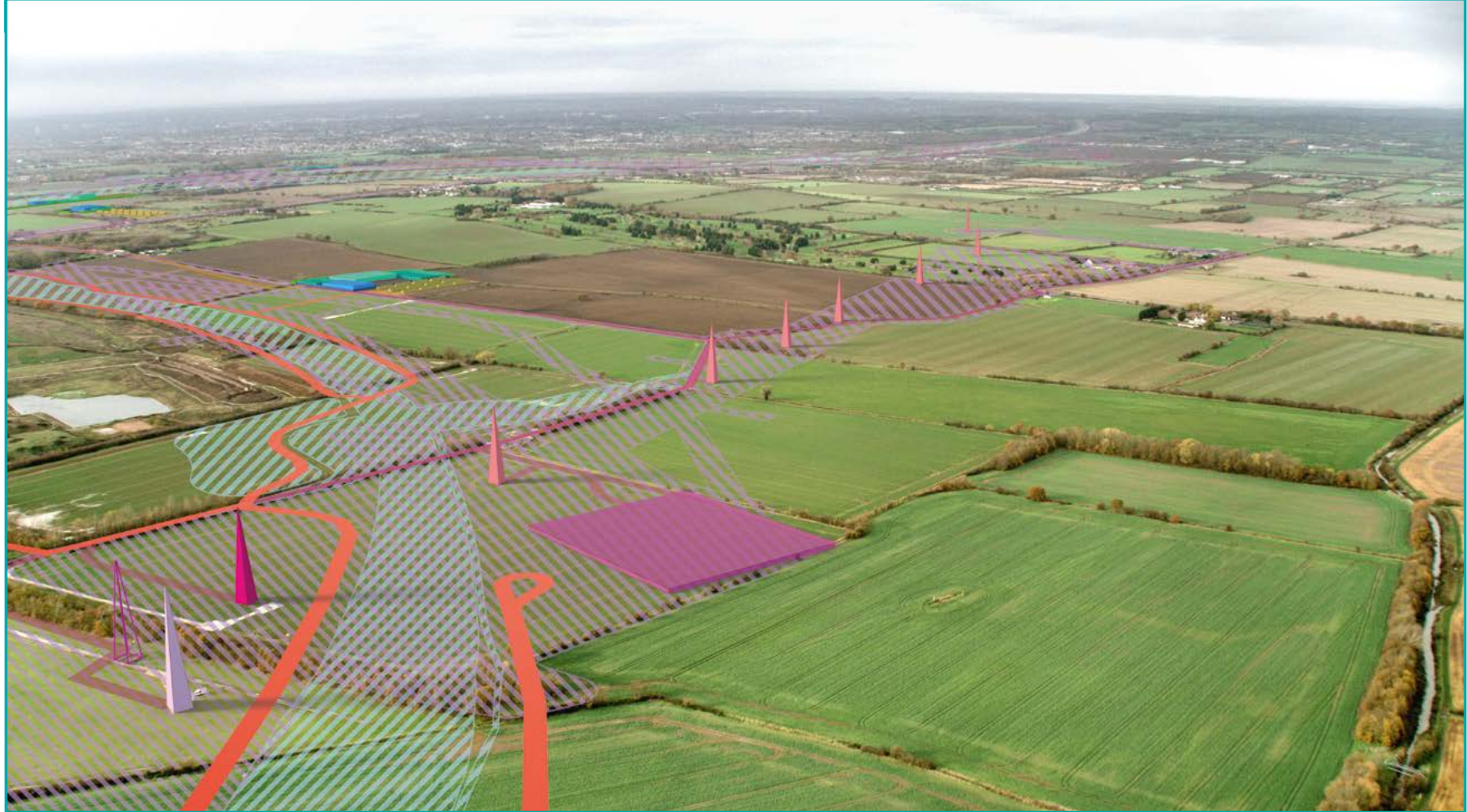
Figure 8-28 Indicative view during construction of the Mardyke Valley and Veolia landfill site from the south-east, looking north-west towards the M25 and Fen Lane, showing Medebridge Compound, Medebridge Utility Logistics Hub and combined utilities and highway construction areas
