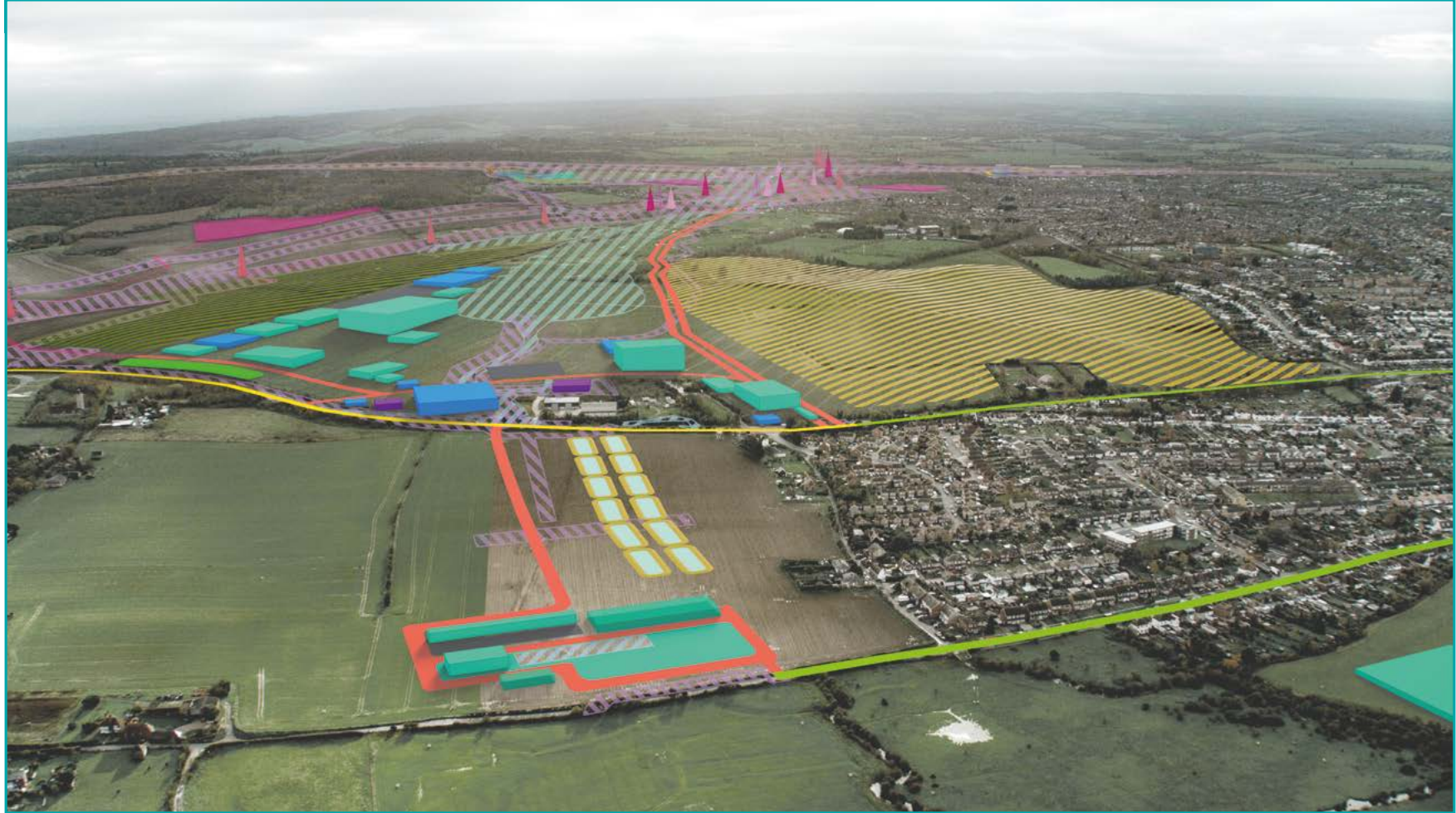
Figure 8-8 Indicative view during construction of the South Tunnel Entrance Compound site from south of Chalk, looking north, showing the South Tunnel Entrance Compound, A226 Gravesend Road compound, Shorne Ifield Road Utility Logistics Hub and combined utilities and highway/tunnel construction areas
