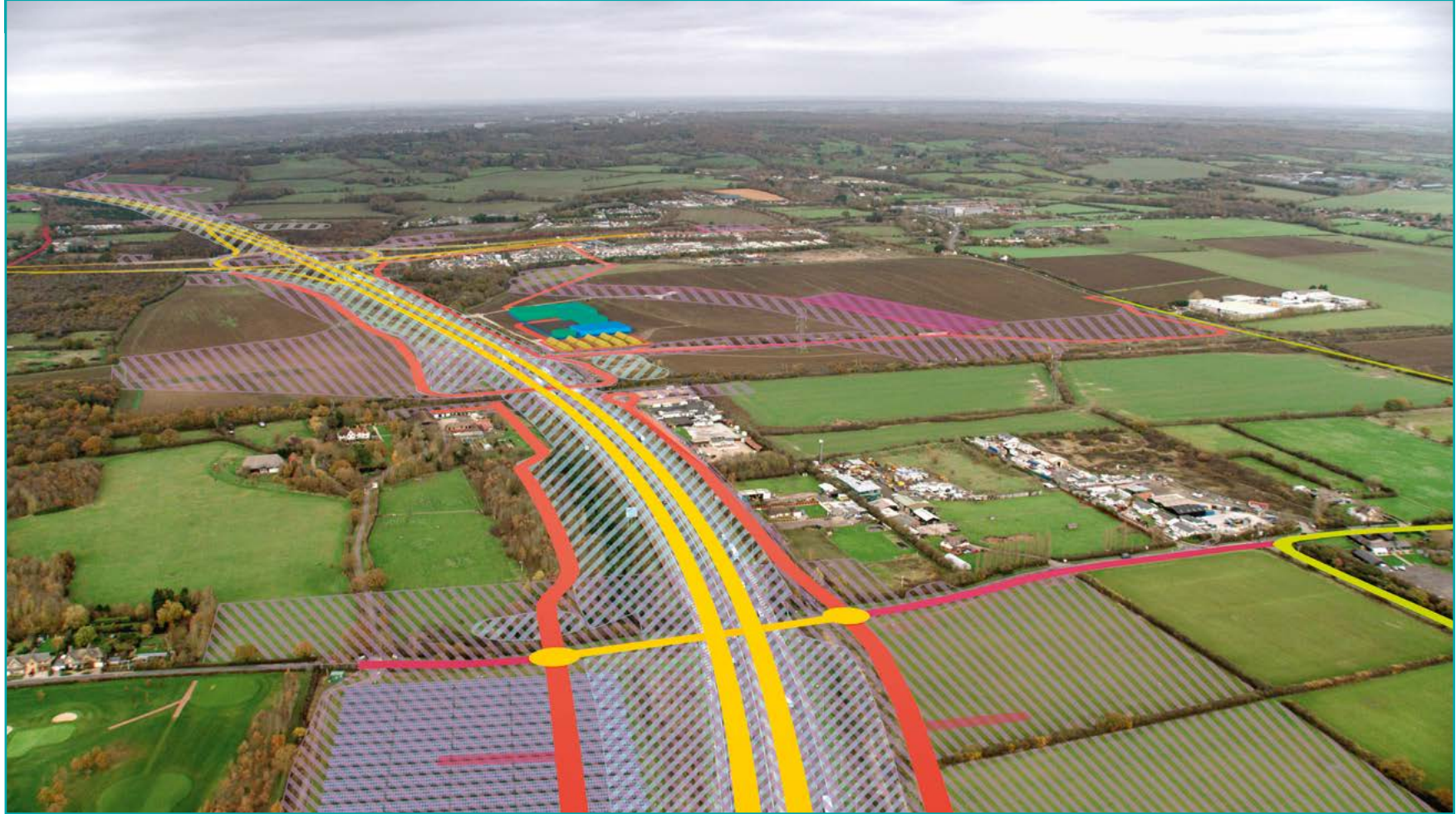
Figure 8-34 Indicative view during construction of the M25 corridor and Saint Mary's Lane from the south, looking north-east towards Wyngray Farm and M25 junction 29, showing the Warley Street Compound, Warley Street Utility Logistics Hub and combined utilities and highway construction areas
