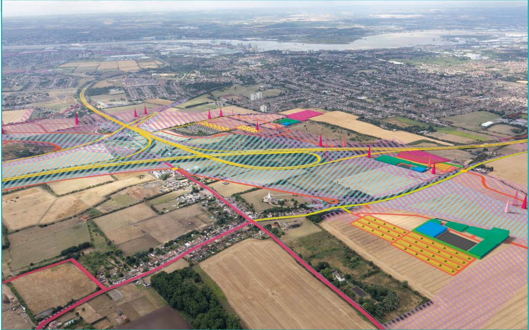
Figure 8-26 Indicative view during construction of the A13 Junction and Baker Street from the north, looking south-west towards Little Thurrock, showing Stifford Clays Compound East and combined utilities and highway construction areas
