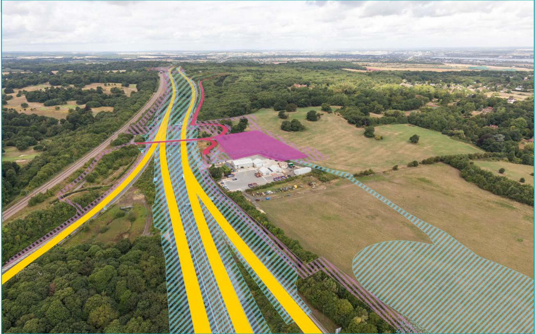
Figure 8-2 Indicative view during construction of the A2 corridor from east of Brewers Road, looking west, showing the Park Pale Lane Utility Logistics Hub and combined utilities and highway construction areas
