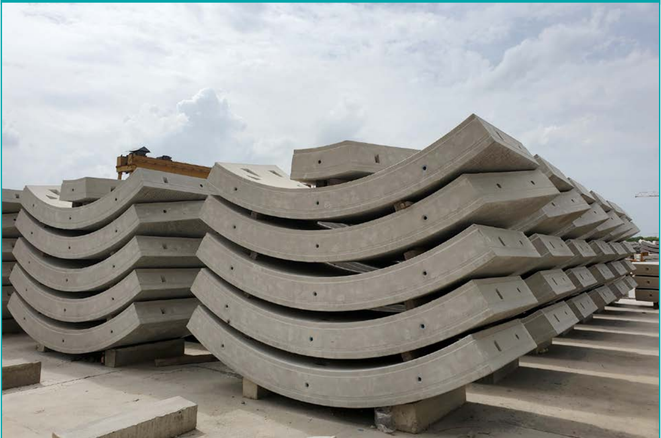
Figure 2-12 Precast concrete tunnel segments
