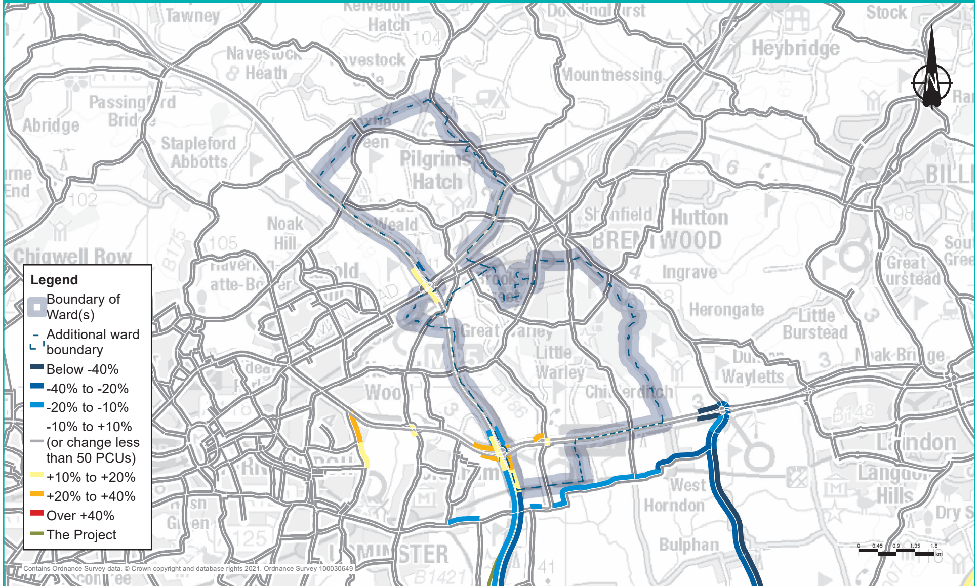
Figure 23.7: Predicted percentage change in traffic flows with the project during the interpeak period in 2029
