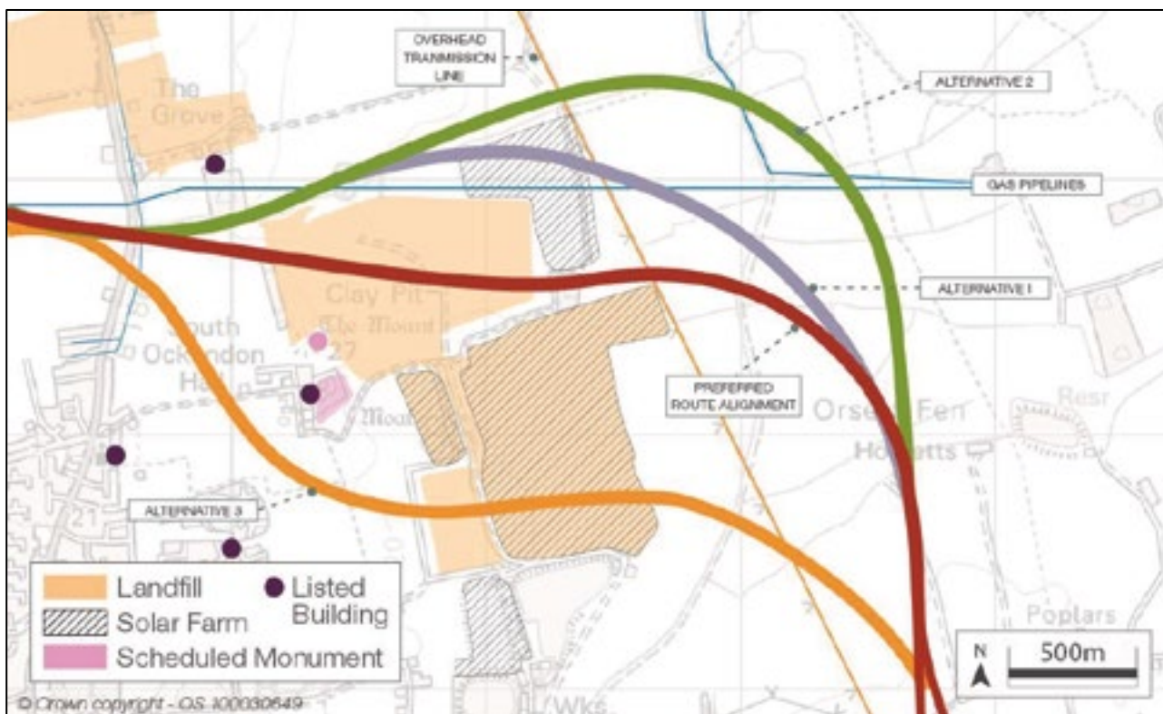
Figure 15.9 Alternative routes at Ockendon Landfill
