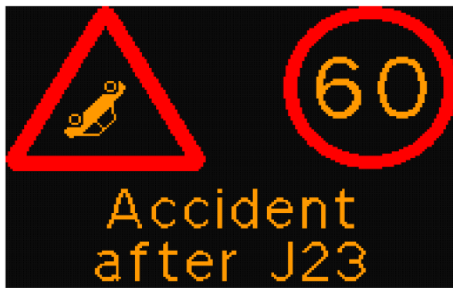
Figure 4f: Variable message sign displaying queue caution information with a reduced mandatory speed limit
