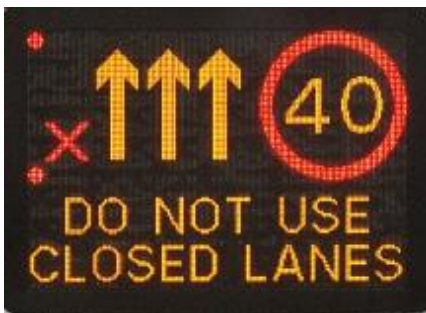
Figure 4g: Variable message sign with lane closure 'wicket' and flashing red lanterns warning of a closed lane
