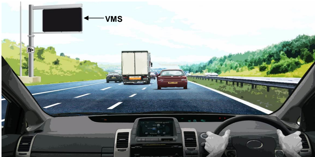
Figure 4B: Illustrative M6 J2 to J4 smart motorway scheme section operating in normal motorway conditions with a blank cantilever mounted VMS
