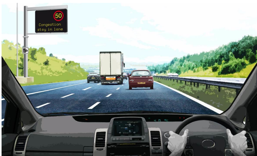
Figure 4D: Illustrative M6 J2 to J4 smart motorway scheme section operating with variable mandatory speed limits and information for road users.
