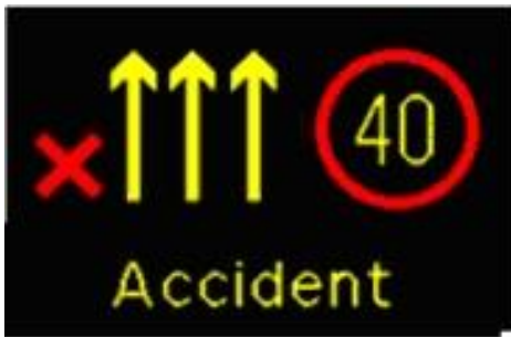
Figure 4G: VMS warning of a closed lane ahead due to an accident
