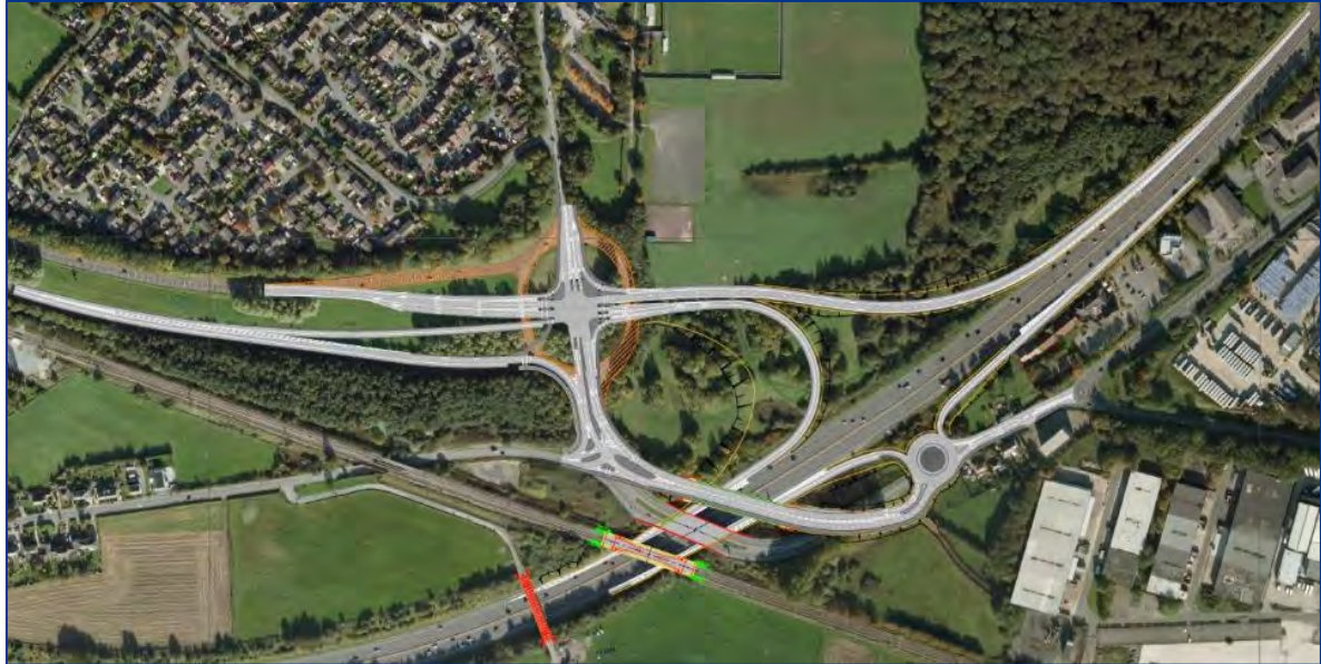
Figure 2-4: Option B – Signalised crossroads layout
