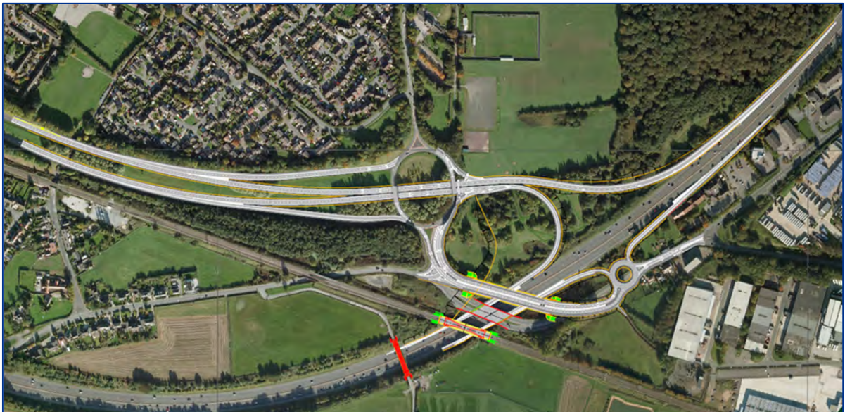
Figure 2-3: Option A - Through-about layout
