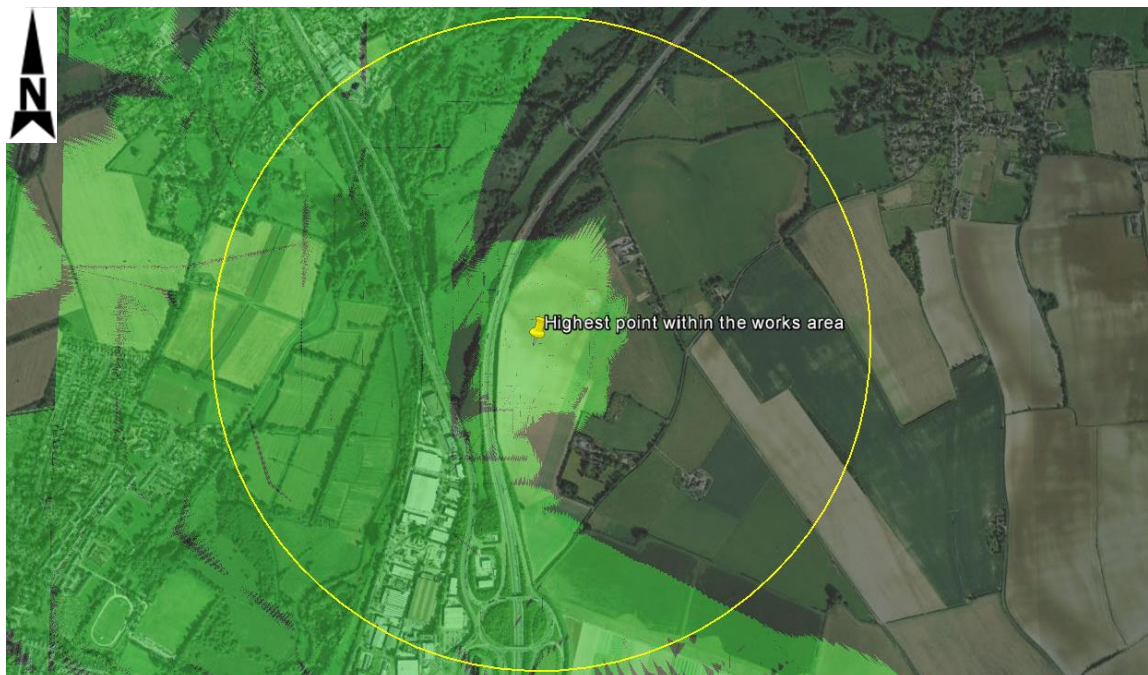
Figure 7-12: Theoretical visibility of an object 12 m high on Easton Down. Map Data: Google, Infoterra Ltd & Bluesky
