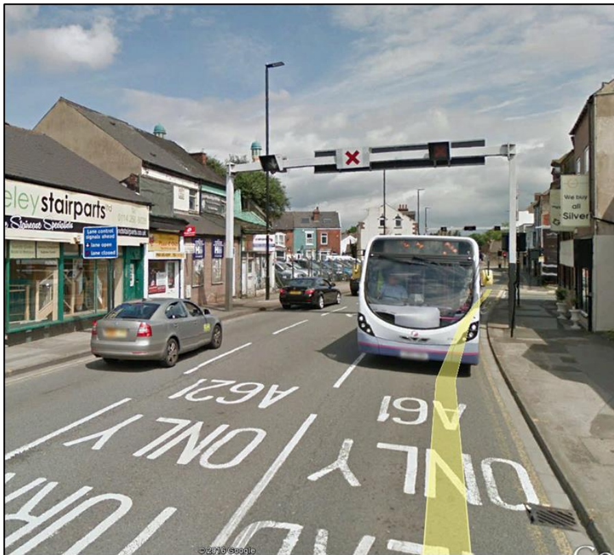
Figure 18-1: Example of Tidal Flow arrangement in Sheffield (#1)
