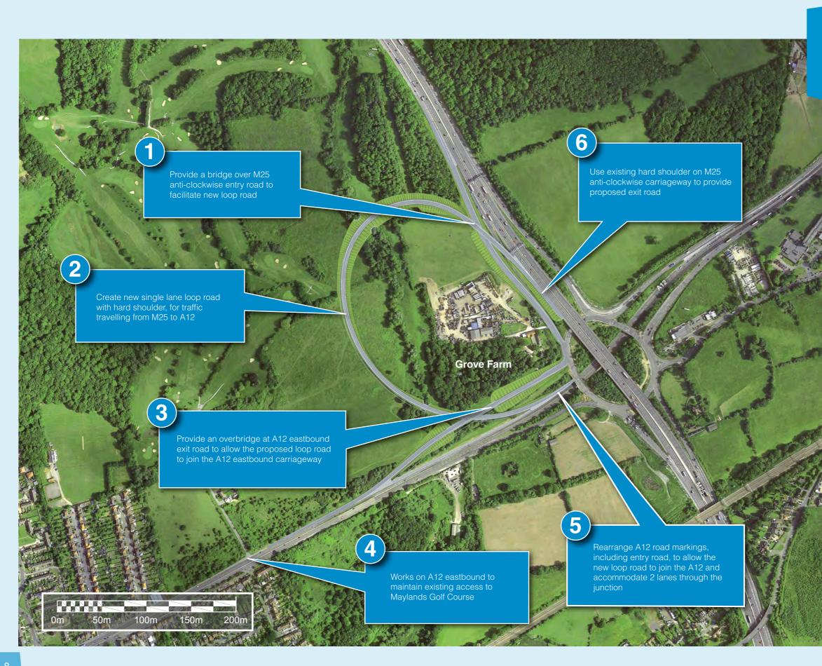
**Option 5C** Single lane loop road, widening of short section of M25
