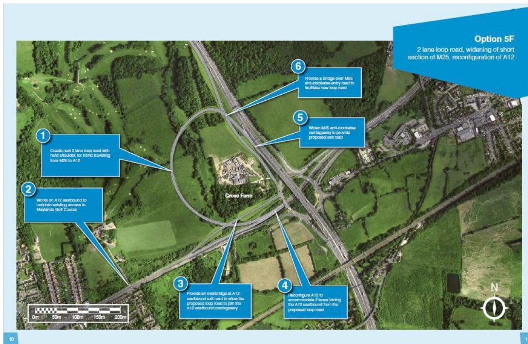
Figure 6: Option 5F – two-lane loop road, widening of short section of M25, and reconfiguration of A12
