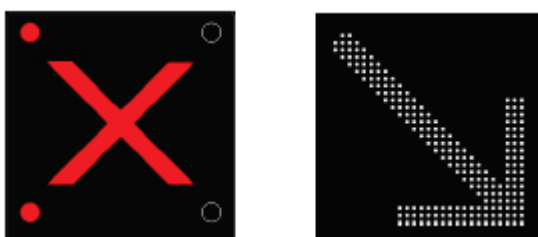
Figure 4e: Red X (do not enter, or proceed in, the traffic lane) aspect with flashing red lanterns and a lane divert signal shown on an advanced motorway indicator over any lane
