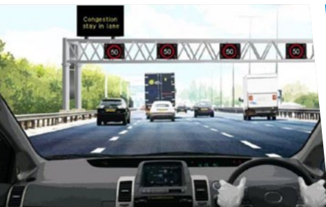
Figure 4c: Illustrative smart motorway All-Lane Running scheme section operating with variable mandatory speed limits.
