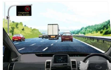
Figure 4d: Illustrative smart motorway All-Lane Running scheme section operating with variable mandatory speed limits and information for road users.
