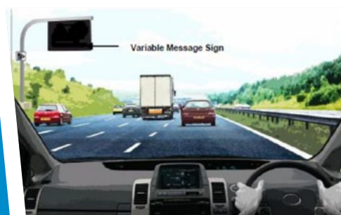
Figure 4d: Illustrative smart motorway All-Lane Running scheme section operating with variable mandatory speed limits and information for road users.
