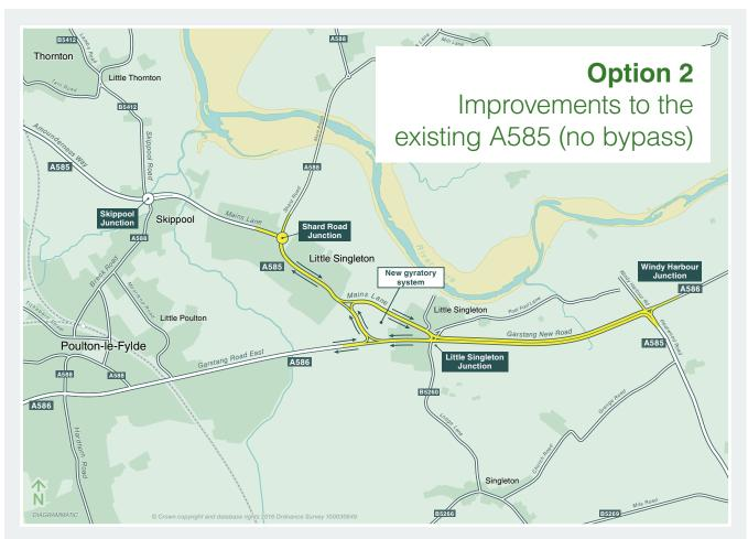
**Option 2: improvements to the existing A585 (no bypass)** – improvements made to the existing road which requires a one way gyratory to be created within and west of Little Singleton. The improvements include making Garstang New Road from Windy Harbour to Little Singleton a dual carriageway, creating a gyratory system within Little Singleton which includes the introduction of a two lane northbound link road and the introduction of a new junction at intersection of Shard Road with Mains Lane.
