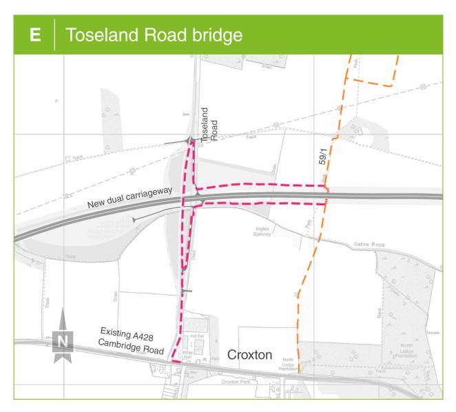
Footpath 59/1 will be diverted. People will cross the dual carriageway using the new Toseland Road bridge. A new route will be created along the south side of the new dual carriageway to connect to the existing footpath to Croxton.
