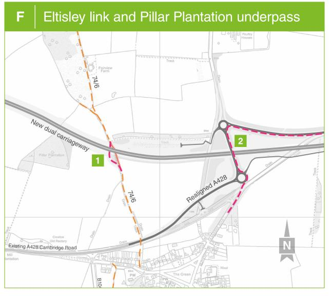
1 We are maintaining access to bridleway 74/6 via a new route. The bridleway will be diverted under the new dual carriageway via an underpass to the west of its existing route. 2 At Eltisley, we will provide a new combined cycleway/ footway at road level and over the new St Ives Road bridge.
