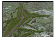
It is now below that of the existing roundabout. The main carriageway would pass through what is, at present, the centre of the Kingsway roundabout.
