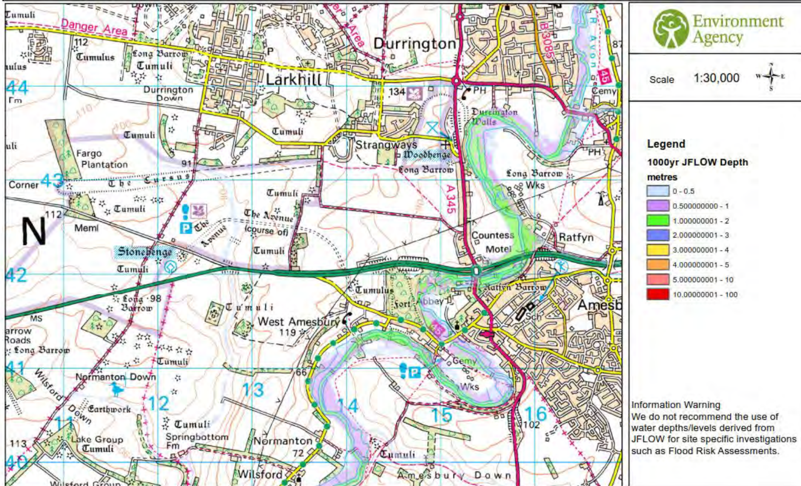
52288 WX - River Avon Fluvial Water depths (m) Without Flood Defences. 1000 year (0.1% AEP). JFLOW Grid Map centred on land at - created 1st August 2017
