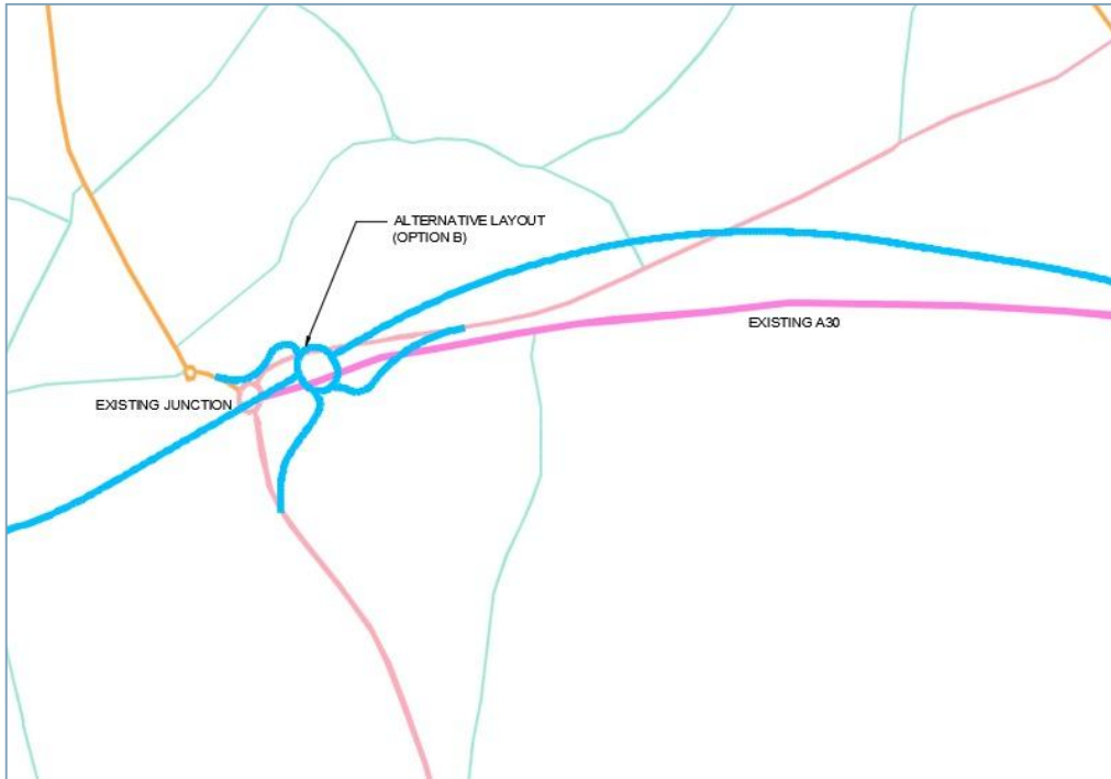
Figure 7-3: Chiverton junction - large gyratory close to existing junction
