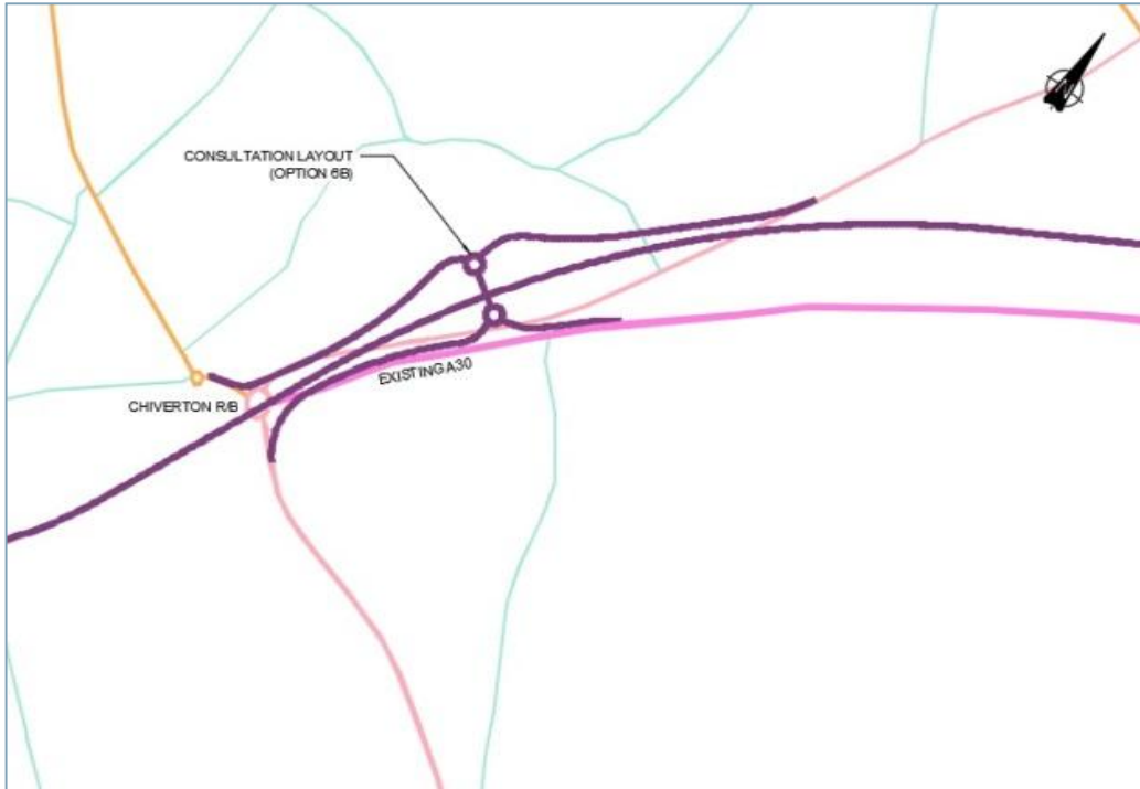
Figure 7-2: Chiverton junction - alternative large gyratory layout
