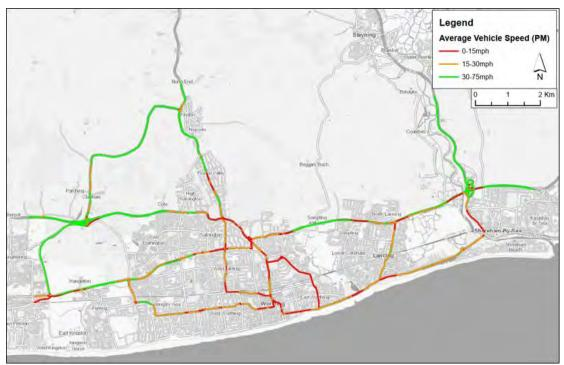
Figure 2-11: Average vehicle speeds in the PM period
