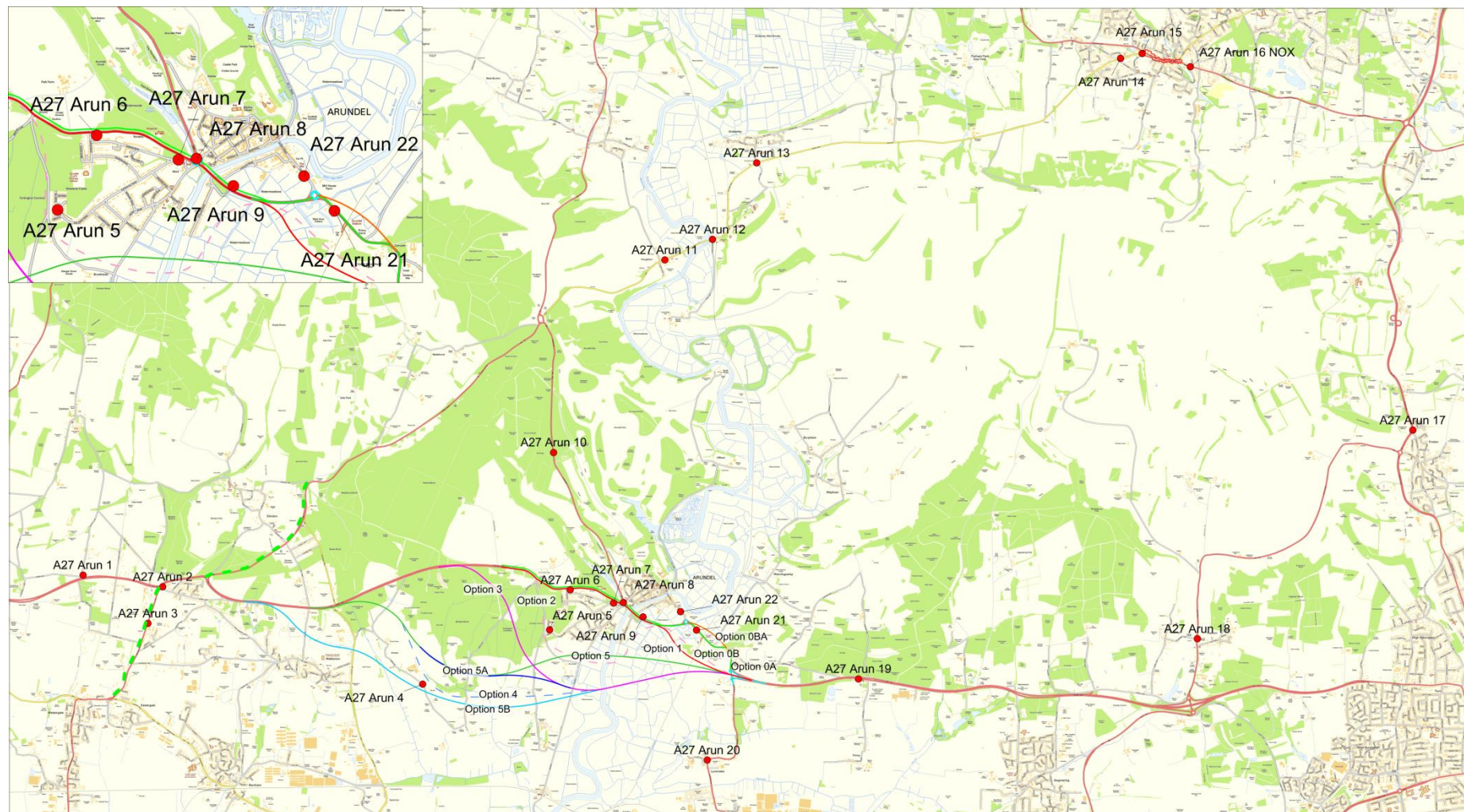
Figure 5-1: Project specific diffusion tube monitoring showing diffusion tube locations and scheme options. PCM links are shown as green dashed line.
