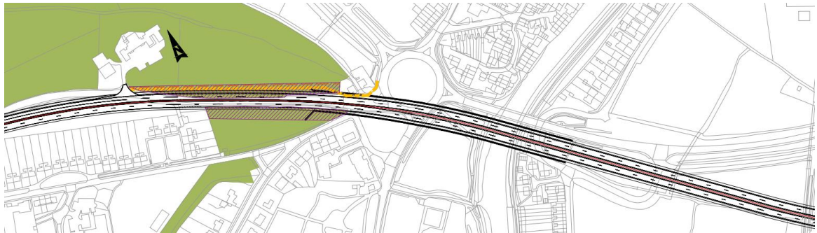
Figure 10-7 Concept layout - flyover with no slip roads
