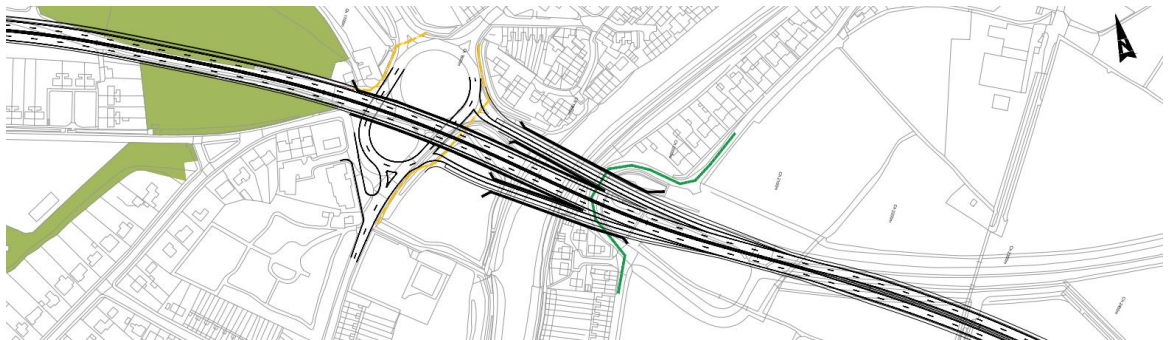
Figure 10-6 Concept layout - flyover with two slip roads
