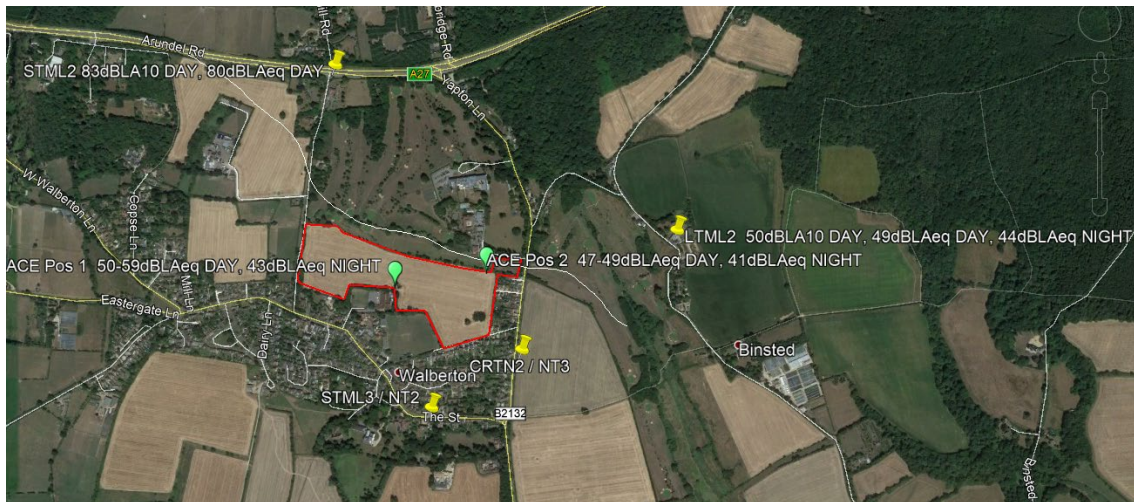
Figure 4.1 Highways England and Ardent Monitoring Positions
