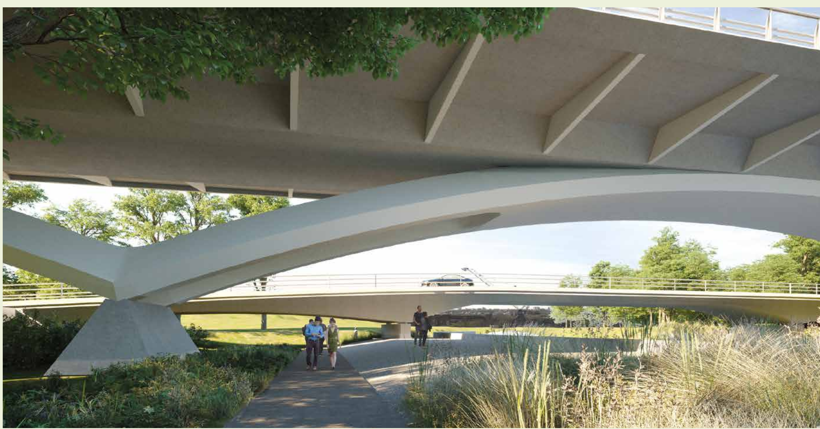
Flyover Cyan (Option 1V5) – Spans over the existing roundabout. The higher profile allows more natural light through and is a less intimidating space for users. The height of the bridge will be similar to the upper levels of nearby buildings.
