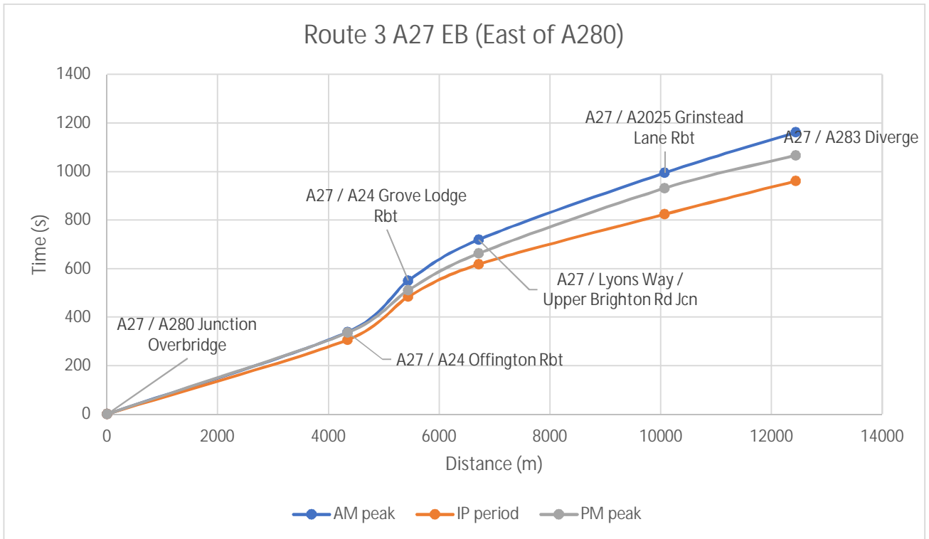
Journey time/distance graph for Route 3 –A27 between Long Furlong and A27/A283 diverge:
