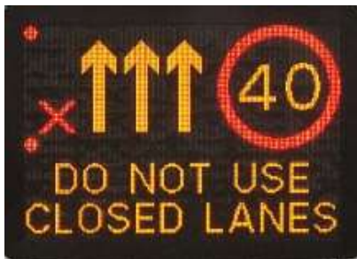
Figure 4g: Variable message sign with flashing red lanterns warning of a closed lane
