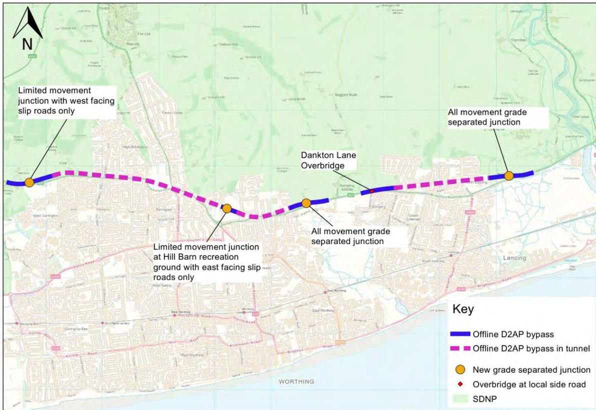
Approximately 4.3km of the route would be underneath ground level on the alignment of the existing A27. The remaining 5.4km would be situated in close proximity (300m or less) north of the existing A27. The majority of the existing A27 carriageway would be retained and adopted as a local access road. This option includes three separate bored tunnel sections approximately 6km long in total throughout the route.
